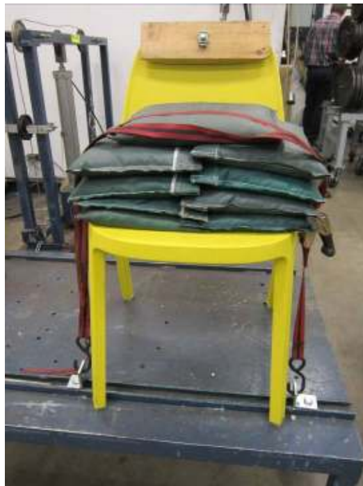
BACK DURABILITY TEST-CYCLIC – SAMPLE – YELLOW
