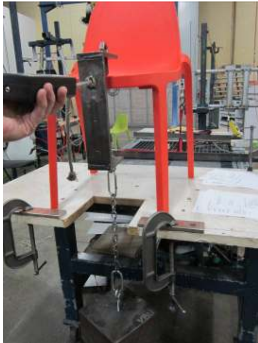
Stability Test – Front – Sample – Orange
