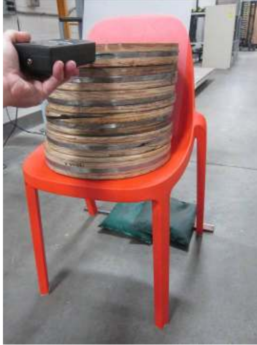
Stability Test – Rear- Sample – Orange
