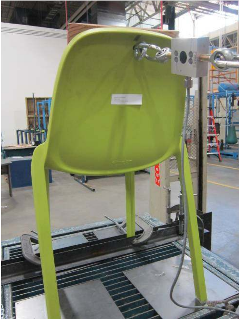
BACK STRENGTH PROCEDURE – STATIC – SAMPLE – Green
