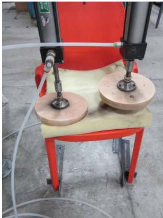
LOAD EASE TEST – SAMPLE - ORANGE
