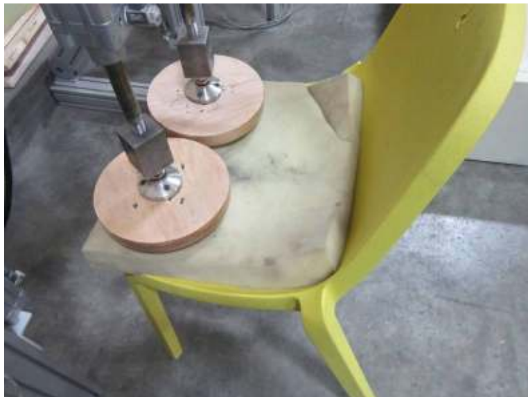
LOAD EASE TEST – SAMPLE - YELLOW
