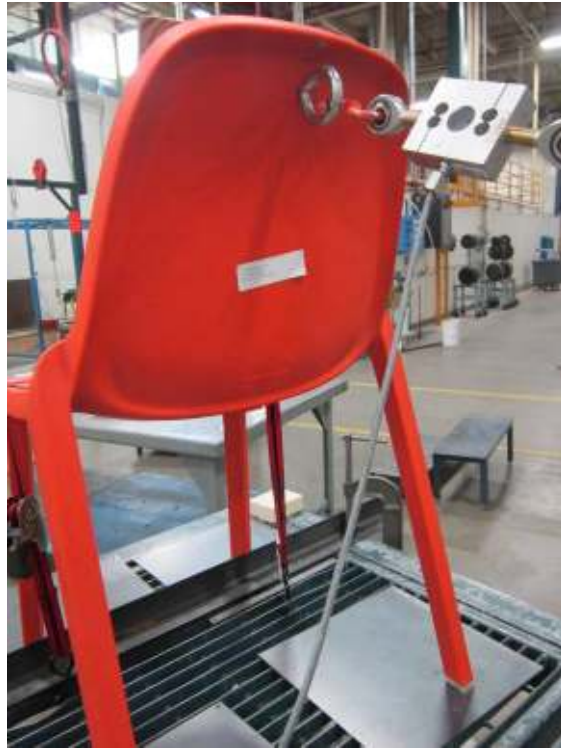
BACK STRENGTH PROCEDURE – STATIC – SAMPLE – ORANGE
