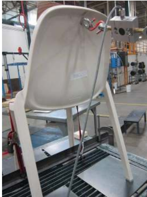
BACK STRENGTH PROCEDURE – STATIC – SAMPLE – WHITE
