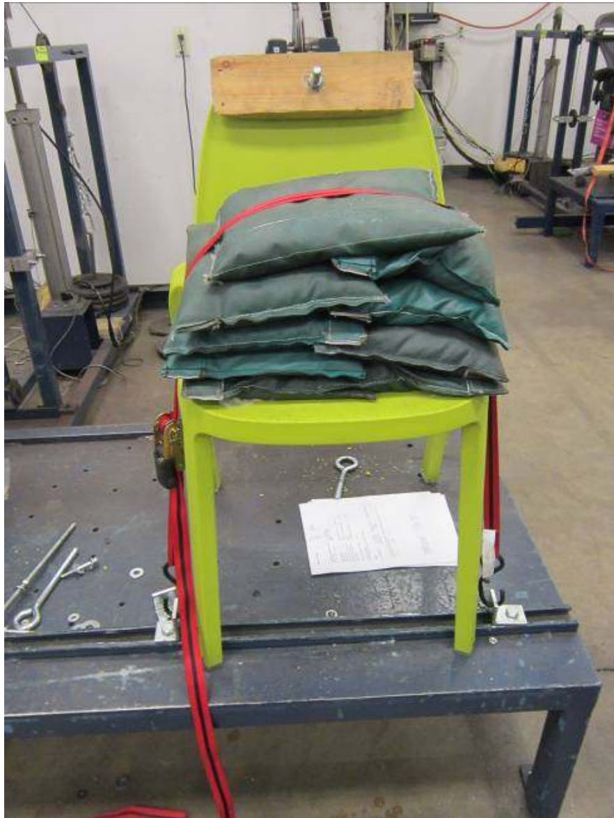
BACK DURABILITY TEST-CYCLIC – SAMPLE – GREEN
