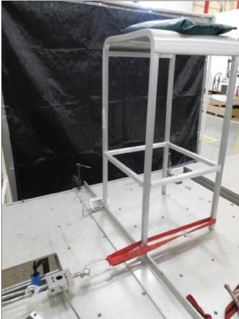
Leg Strength Test – Side Application
